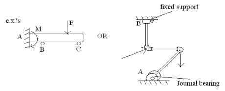
Redundancy is generally good, but it creates too many unknowns for our 3 (2D) equations or 6 (3D) equations of static equilibrium. Note how most of the examples throughout this chapter have used primarily pins or rollers, because multiple fixed supports  $\Rightarrow$  redundancy.
