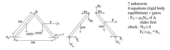
$\label{eq:constraint} \begin{array}{l} OR\\ \text{-} F_C = \mu_C N_C \text{, if } C \text{ slides first}\\ \text{check:} \ N_A \geq 0\\ F_A \leq \mu_A \ ^* N_A \end{array}$
