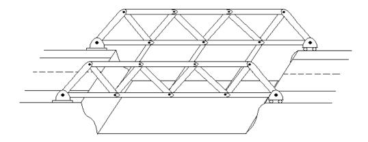
The load from the road and vehicles rests entirely on the beams, as we can see in the exaggerated diagram. The beams are connected to the bottom joints of the trusses, so the load is transferred entirely to those bottom joints. Our assumption is thus valid. Finally, the truss rests on the ground at each end of the valley, so the load is entirely transferred to the ground. The beams connecting the top joints of the trusses are not shown but typically would be present.
