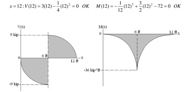
note: w(x) from  $6^+ \le x \le 12$  is  $\frac{1}{2}x - 3$  NOT just  $\frac{1}{2}x$  because our origin is at the far left side of the beam, not the middle of the beam.
