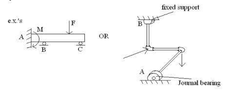
Redundancy is generally good, but it creates too many unknowns for our 3 (2D) equations or 6 (3D) equations of static equilibrium. Note how most of the examples
