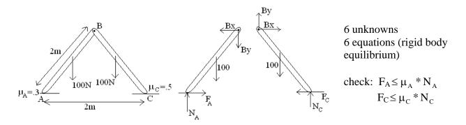
2) Maximizing an external force (minimizing an angle); *all* contact points on the verge of slipping.
