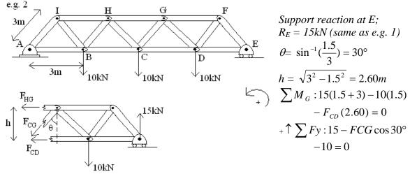
$$\xrightarrow{+} \sum Fx : -F_{HG} - 5.77 \sin 30^{\circ} -20.2 = 0 F_{CD} = 20.2kN(T) \qquad F_{CG} = 5.77kN(T) \qquad F_{HG} = -23.1 = 23.1kN(C)$$
