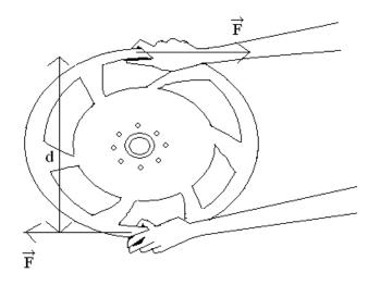
The shaft pictured below could be *anywhere* on the wheel and would have the same moment about its axis (as long as it is perpendicular to the wheel). The moment would be less than Fd for an axis not perpendicular to the wheel.
