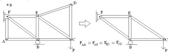
If three elements meet at a joint, two of which *are* collinear, and there is no external force at that joint, then the third member is a zero-force member.
