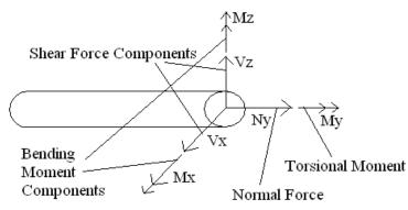
note: The sense of V and M drawn to the left and above is treated as positive in structural engineering.
