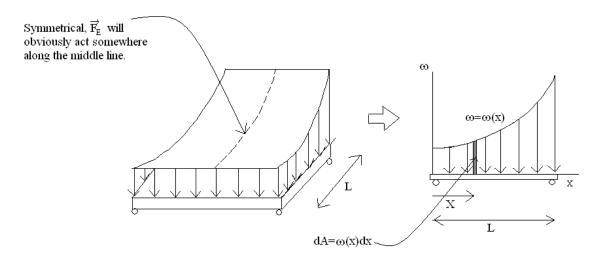
$$F_{R} = A = \int_{L} \omega(x) dx \qquad M_{RO} = \int_{L} x \omega(x) dx$$
