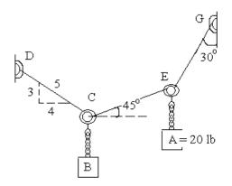
Draw a free body diagram at E and solve for  $T_{EC}$  and  $T_{EG}$ . Then, draw a free body diagram at C and solve for  $T_{CD}$  and  $W_B$ .
