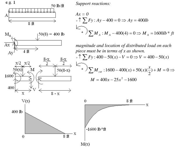
note: Fixed beams like this are sometimes tapered (thicker near the support) in order to be cost effective, since we can see that the forces are large only near the support.
