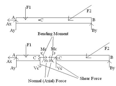
Nc is an axial (tensile or compressive) force, which is a type of force we've already dealt with. Note equal and opposite forces on each piece of the beam, from Newton's 3<sup>rd</sup> Law.
