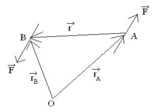
O is an arbitrary point in space The two  $\vec{F}$  forces are located in the same plane and are of equal magnitude.
