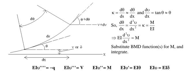
q, V, M should be non-zero constant, or functions of x (If non-prismatic beam, then I also depends on x)
